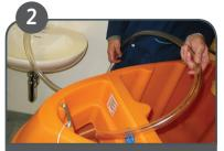
Fill solution tank with clean water.
