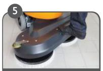
Position tool(s) precisely under the lifted brush unit.
