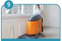
Clean the floor. When re-filling the tank and after use always switch off the machine with the key switch.
