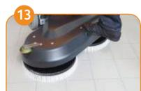
Remove tools with foot pedal (while brush unit is in upper position).
