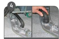
Mount squeegee with 'click' mechanism and attach the suction hoses on both sides.
