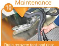
Drain recovery tank and rins with fresh water, then drain
