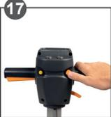
**17** Press orange button and move into upright position to lock handle for parking/storage.
