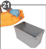
**21** Open and remove clear recovery tank cover. Empty and rinse.
