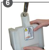
**6** Fill white solution tank with clean water. Dose cleaning product into solution tank.
