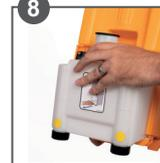
**8** Refit white solution tank into orange cover tank and refit into machine.
