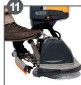
**11** Disengage parking/ storage mode using foot pedal.
