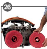
**26** Clean and rinse and replace brushes/pad drives/pads. Replace pads as needed.
