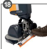
**18** Disengage squeegee by lifting up squeegee with foot.
