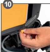
**10** Set both water flow levers for application. 5 settings from low to high (-) or (+).
