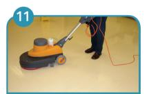
Commence buffing / spray cleaning at furthest point from plug socket. Work backward with cable behind you at all times.
