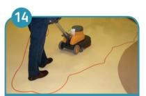
Turn away from the socket at the end of each pass so cable lies on the area already cleaned. Allow 2" overlap.
