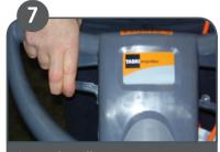
Lower handle to a comfortable position by squeezing lower lever.
