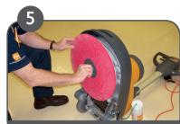
Tip machine back to put handle on floor and fit pad. Turn pad retainer anticlockwise to lock on.
