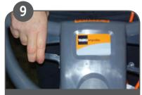
Lower handle to a comfortable position by squeezing lower lever.
