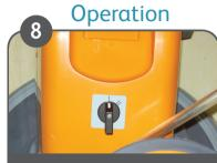
Ensure speed control switch is in first position (low speed).
