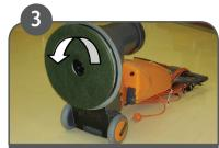
Tip machine back to put handle on floor and fit pad/ pad drive or brush.
