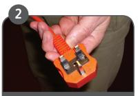
Check equipment, especially plug and cable. Report any fault or damage to a supervisor. Label as faulty and do not use.
