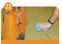
Wind cable back into handle, wiping clean with a damp
