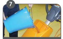
For wet scrubbing fill tank or mop cleaning solution on floor as appropriate.
