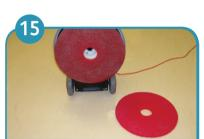
Check pad/brush regularly for clogging. Unplug machine and turn/change pad as required.
