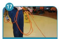
When changing socket, coil cable from machine to plug, not plug to machine, to avoid twisting.
