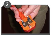
Check equipment, especially plug and cable. Report any fault or damage to a supervisor. Label as faulty and do not use.
