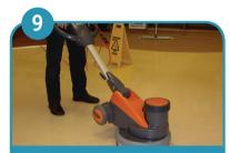
Commence buffing/spray cleaning at furthest point from plug socket.
