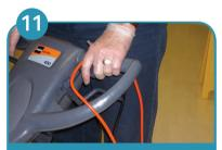
Hold cable over handle, NOT over shoulder. Keep cable out of solution.
