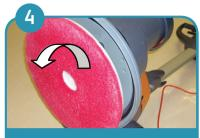
Tip machine back to put handle on floor and fit pad/pad drive or brush.
