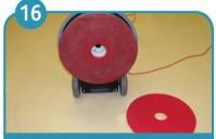
Check pad/brush regularly for clogging. Unplug machine and turn/change pad as required.
