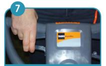
Squeeze lower lever. Adjust handle position so operator's back is straight with arms slightly bent. Release lever to lock in position.
