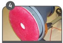
Tip machine back to put handle on floor and fit pad/ pad drive or brush. Raise back upright..
