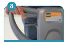
To activate machine hold locked handle so pad is flat to floor. Press orange safety button and squeeze upper lever.
