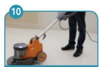
Commence scrubbing at furthest point from plug socket. Work backward with cable behind you at all times.
