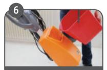
For wet scrubbing fill tank or mop cleaning solution on floor as appropriate.
