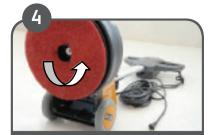
Tip machine back to put handle on floor and fit pad/pad drive or brush. Raise back upright.
