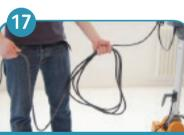
When changing socket, coil cable from machine to plug, not plug to machine, to avoid twisting.
