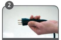
Check equipment, especially plug and cable. Report any fault or damage to a supervisor.
