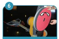
Tip machine back to put handle on floor and fit pad. Turn pad retainer anticlockwise to lock on.
