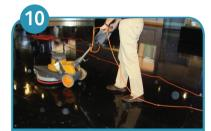
Turn away from the socket at the end of each pass so cable lies on the area already cleaned. Allow 2" overlap.
