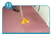
At end of pass release trigger and continue backwards for a few inches to recover last drops of water.
