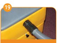
Switch off vacuum and detach hoses ensuring no dirty water escapes from the extraction hose.
