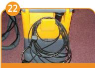
Wind cable back wiping clean with damp cloth and checking as you do.
