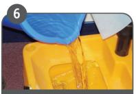
Fill solution tank with clean water and appropriate detergent dilution. Ensure lid is fitted correctly.
