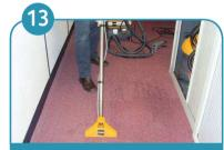
If necessary, pass over same path again without squeezing the trigger to ensure maximum water removal.
