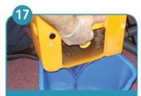
Stop immediately and empty recovery tank. (Pull black release button to remove tank).
