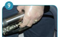
Holding the wand head flat to the floor, squeeze trigger to release solution.
