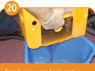
Empty recovery tank and clean (tank may be removed
