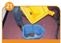
Empty solution tank and clear fluff and debris from wand.
