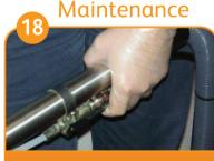
Switch off pump and operate trigger to release pressure.
