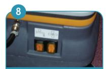
Switch on water (trigger may need to be operated to release airlock and allow solution to spray.)
