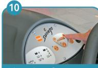
Adjust solution flow. (depending on model - with buttons on dashboard or with lever).
