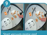
Start vacuum motor and solution supply (press orange buttons).
