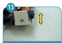
Front squeegee for removing the water when going backwards. Use the lever right-hand!
