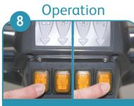
Turn machine on (left button), and start solution supply (right button).
