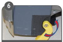
Release parking position by lifting machine a bit (parking position is flipped back automatically).
