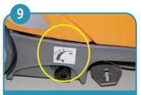
Adjust solution flow manually.
