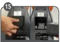
Remove battery by pressing release button
