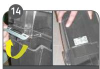
Remove tank from machine by pulling the hook. Unlock and remove filter housing. Empty tank and rinse both tanks
