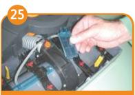
Rotate yellow clip. Remove transparent converter cover. Check suction conveyor that it is free from debris. Remount cover and book it
