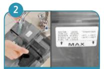
Fill solution tank with fresh water up to indicated mark. Label with mark is on solution tank side.
