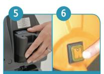
5. Add fully charged battery to the machine, make sure you hear a "click"
