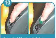
Press first black switch for suction and afterwards water pump switch (green lamp lights up)
