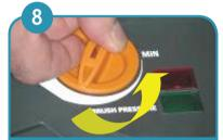
Adjust brush pressure by turning knob slowly anticlockwise until red light turns off. Red light indicates that motor is overloaded.
