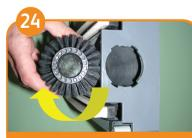
Check bristle length before reinstall brush roller. Refit brush holder and turn it clockwise until lock latches into place.
