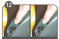
Switch off water pump. Run suction unit for 10 seconds more to suck out remaining water. Switch off suction motor
