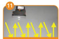
If red light goes on and off immediately while working, adjustment is correct.
