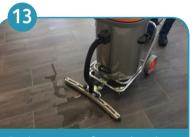
Push vacumat forward and make sure the cable is lying flat on the dry floor.
