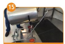
Remove filters and empty the machine.
