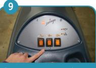
Start vacuum motor and solution supply (press orange buttons).
