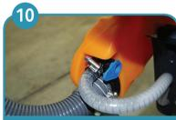
Adjust solution flow. (with blue lever)
