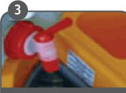
Dose cleaning product into dosing aid, then pour it into the solution tank.
