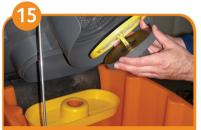
Remove the floating unit (filter and floater) with a rotation of the yellow filter in anticlockwise direction.
