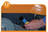
Clean solution filter and put it back into machine.
