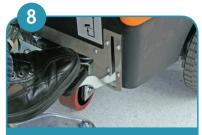
Lower brush unit with foot pedal. The brush will then be coupled automatically.
