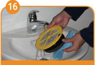
Clean the floating unit under running water and put it back into machine.
