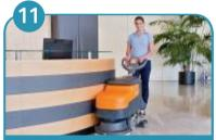
Clean the floor. After that switch off the machine wirth the key switch.
