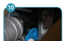
Adjust solution flow with the light blue lever on the left side of the machine.
