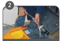
Fill solution tank with clean water.
