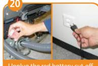
Unplug the red battery cut-off plug, then plug in the cable of the battery charger.
