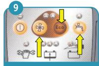
Start vacuum motor and solution supply (press orange buttons)
