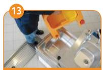
Rinse the recovery tank with fresh water. To do so it can be removed from the machine.
