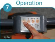
To turn on the machine press the start button for 3 seconds.
