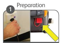
Unplug cable of battery charger, then plug red battery cut-off plug into the machine
