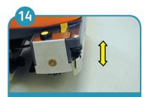
Front squeegee for removing the water when going backwards. Use the lever right-hand!
