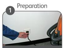
Unplug cable of battery charger, wind up and place on machine (holder).
