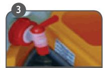
Dose cleaning product into dosing aid, then pour it into the solution tank.
