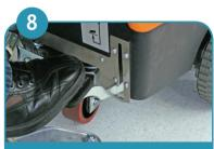
Lower brush with foot pedal OR press brush button on display.
