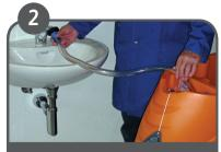
Fill solution tank with clean water.
